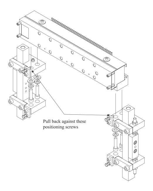
The magnet rack must be adjusted in two directions, horizontal and vertical.
