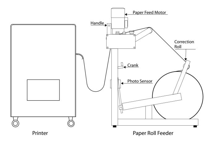
To operate the Paper Roll Feeder, the main switch on the Printer must be in the "on" position.
