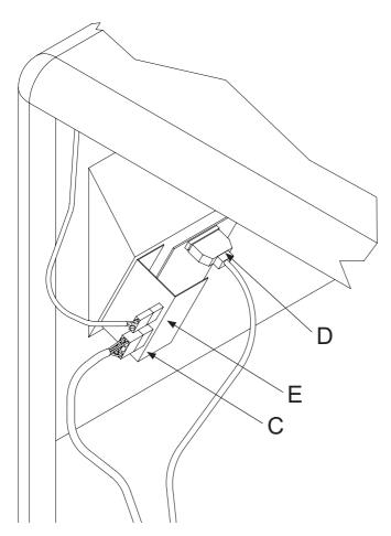
Disconnect the cables to the on/off switch (C), operating panel (D) and safety switches (E). Note that these cables is to be disconnected at the end on the back of the operator panel.
