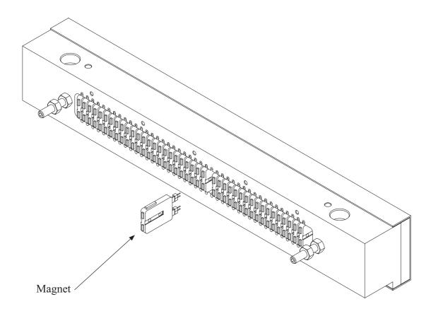
**Step 3.** Check the magnets internal resistance if you have an ohm-meter available. The resistance should be from 185 ohm up to 240 ohm. Any value outside this range indicates a defective magnet.
