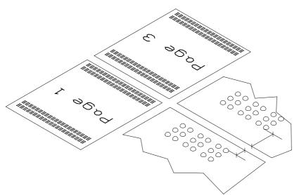
If the paper cutter is moved too far out from the printer, the bottom margin on page one will be to narrower than the top margin on page 3.
