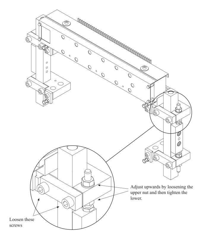
Note! Adjust in small steps, only 1/4 of a revolution at a time. Then test the braille quality.
