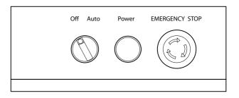
**Note!** If any work is to be done near or at the correction rolls, the switch should be switched to "Off". This will disable the photo sensor, and the feeder motor will not start accidentally.
