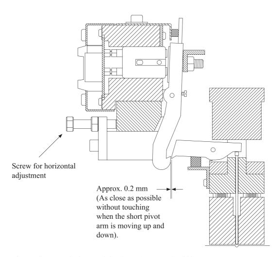
The gap between the long and the short pivot arm should be approx. 0.2 mm.
