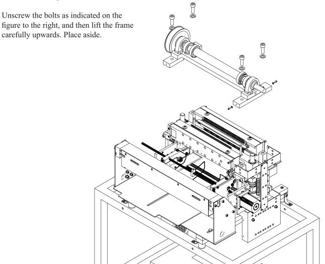
7. Now the beams and paper shoes can be lifted carefully upwards. Assembly is done in the reverse order.
