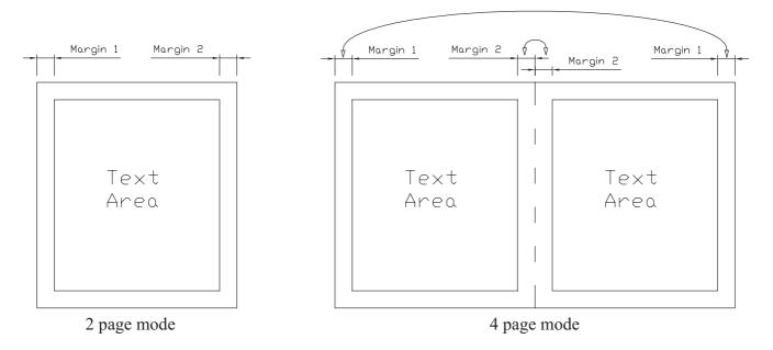
Note when printing in 4 page mode, the value on margin 1 will affect both the "outer" margins. And the value on margin 2 will affect both the "inner" margins.
