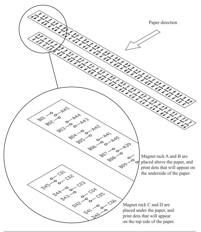
Here the letter "P" means page. The figure shows a sheet of paper printed in "4-page mode". The two circles is showing which magnet that has made the different dots. Line no. one will be in the upper left corner when facing the page.
