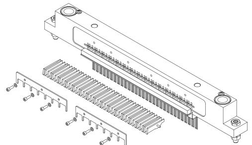
1. Remove the six screws as indicated on the figure. Pull out the short pivot arms, there are 45 pcs. on each side.
