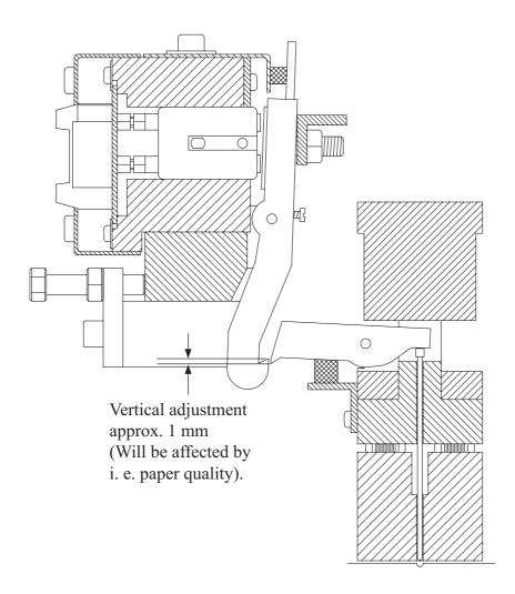
The vertical adjustment of the magnet rack sets the pressure of the printing pins when making dots.
