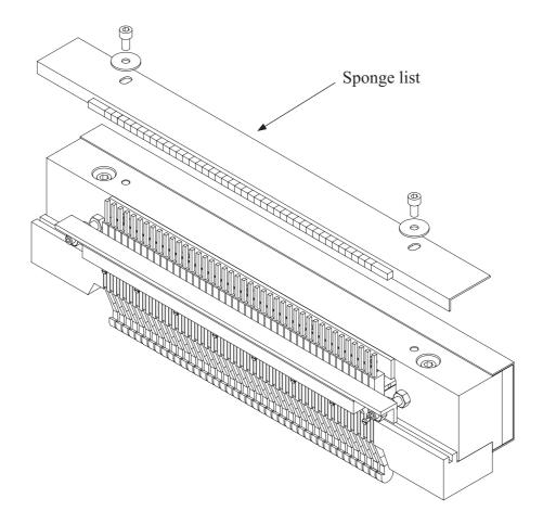
**Step 2.** Remove the two nuts holding the support list, and then remove the support list.
