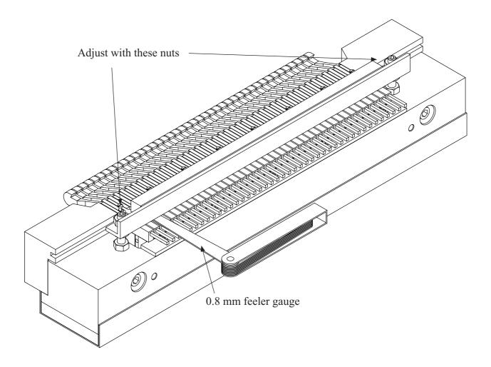
The second adjustment is the pressure the sponge list exerts against the pivot arms. The sponge list works as a return spring for the pivot arms. The correct adjustment is when the sponge list is slightly pressing against the pivot arms, but the pivot arms can still move freely.
