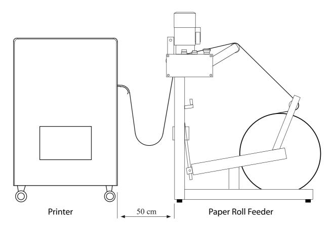
The Paper Roll Feeder may be considered as an independent unit, even though it is switched on and off with the main switch on the Printer.
