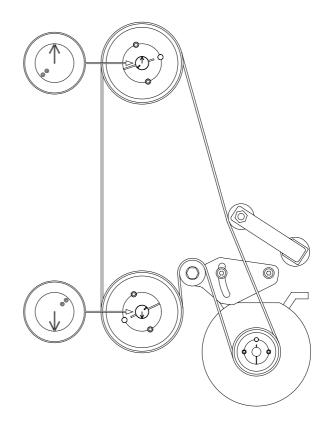
When the arrows at the end of the shafts are pointing in the opposite direction of each other, the short pivot arms will be approx. positioned like in the figure below:
