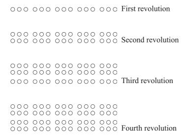
To be able to print interpoint (where both sides of paper are printed simultaneously), the back page is offset a little to the right and a little down to fit in between the dots on the front page. Please see figure below:
