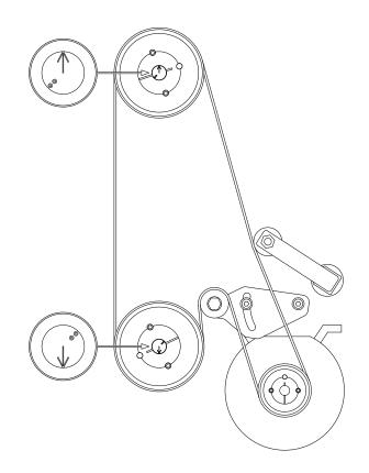
0 Ø When the arrows at the end of the shafts are pointing in the opposite direction of each other, the short pivot arms will be approx. positioned like in the figure below:
