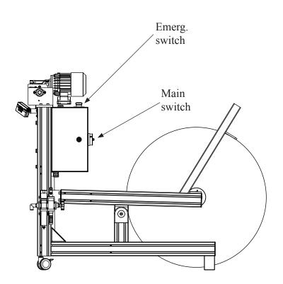
The way the units are connected regarding the 230V is explained in the figure above. Please note that the emergency switch on the Paper Roll Feeder will turn off the power and air to all machines when they are pushed down. The main switch on the Paper Roll Feeder will also turn everything off.
