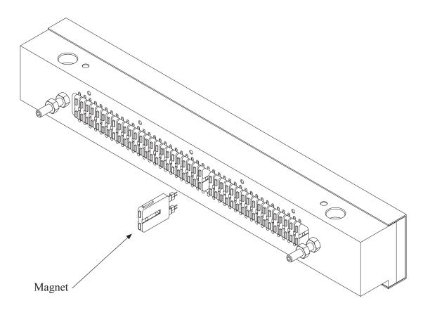
**Step 3.** Check the magnets internal resistance if you have an ohm-meter available. The resistance should be from 185 ohm up to 240 ohm. Any value outside this range indicates a defective magnet.
