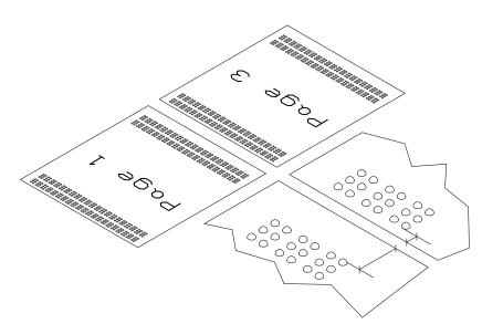
If the paper cutter is too close to the Printer, the bottom margin on page one is bigger than the top margin on page three.
