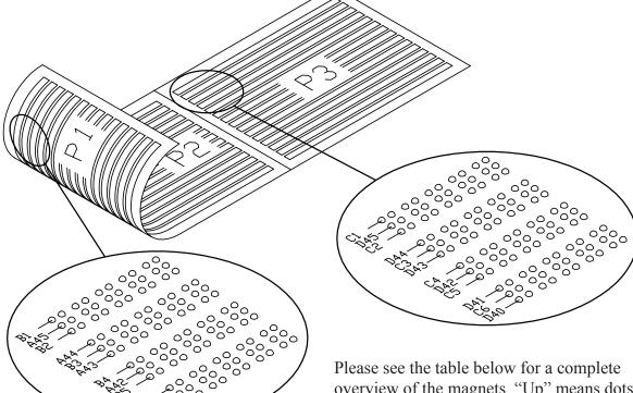
Please see the table below for a complete overview of the magnets. "Up" means dots on top of the sheet, and "Down" means dots on the underside of the sheet.
