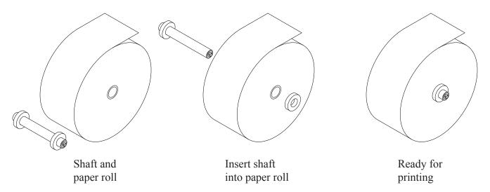
Put the shaft in the center of the roll, and ensure that the shaft is approximately in the centre sideways. Fasten the shaft. The roll must be placed so that the paper is rolled off at the top. (See figure).
