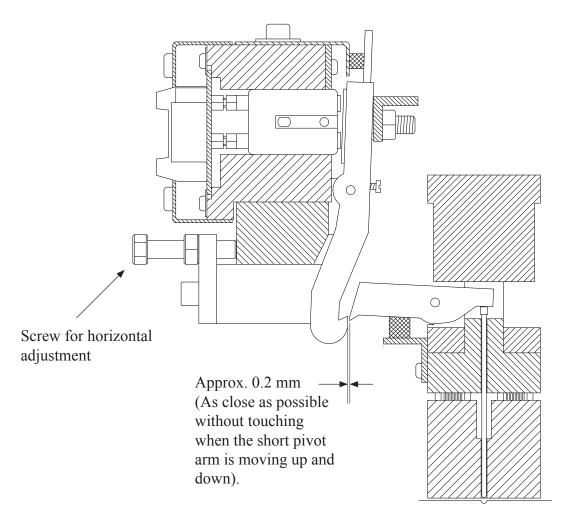
The gap between the long and the short pivot arm should be approx. 0.2 mm. When adjusting this, make sure that the gap is even for all the pivot arms and the same on both ends of the magnet rack.
