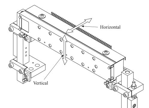
To be able to adjust the magnet rack correctly, it is necessary to put the Printer in "printing position".
