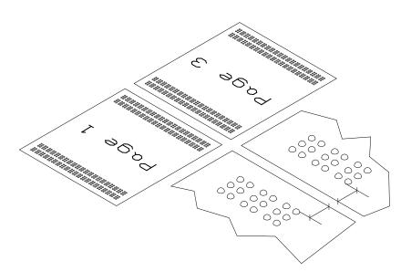
When the paper cutter is correctly adjusted, the bottom margin on page one has approx. the same size as the top margin on page 3. The edge on the sheet is also aligned with the text.
