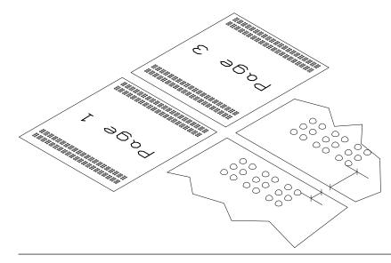
If the paper cutter is moved too far out from the Printer, the bottom margin on page one will be narrower than the top margin on page 3.
