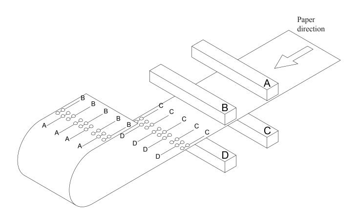
The crossection below is a "theoretical" figure showing the parts inside the printing mechanism. The Printer has been "sliced" to show more detailed of how it is constructed.
