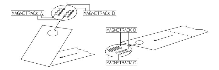
Observe that the same printing mechanism (magnet, long pivot arm, short pivot arm and printing pin) makes all the dots in a column downwards the page.
