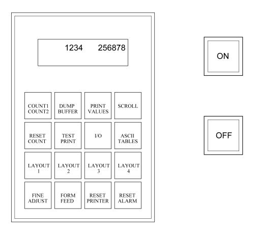
The green switch marked "ON" will turn the printer on, and the red switch marked "OFF" will turn the printer off.
