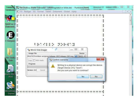
Then press yes and the program will write the firmware to the SD-Card.
