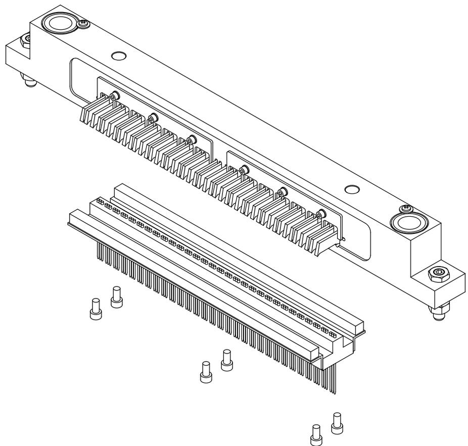
Now defect printing pins can be replaced.
