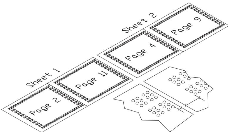
If the paper cutter is moved too far out from the Printer, the right margin on page 11 will be narrower than the left margin on page 4.
