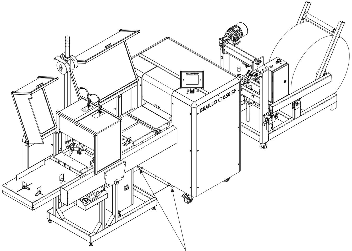
Use these handles to align the S&F unit with the Printer
