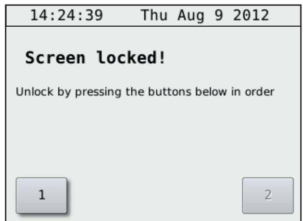
The display screen will automatically lock after a certain amount of time. To unlock press button 1 and then 2.
