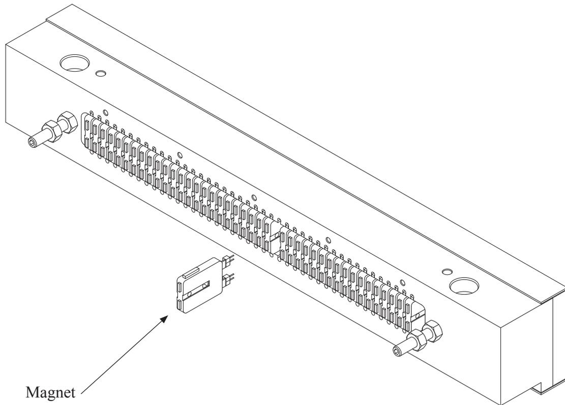
**Step 3.** Check the magnets internal resistance if you have an ohm-meter available. The resistance should be between 185 ohm and 240 ohm. Any value outside this range indicates a defective magnet.
