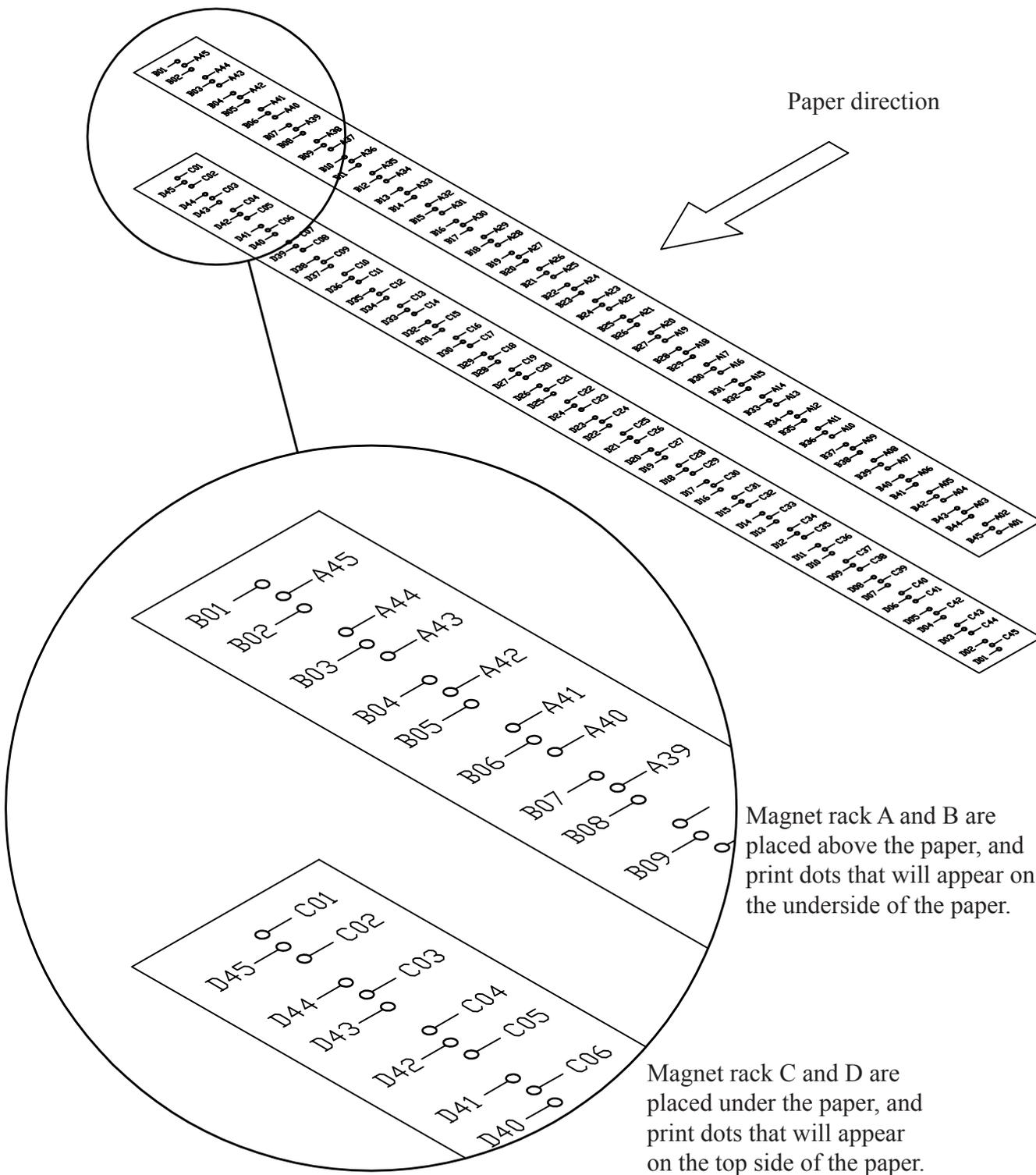
The letter “P” means page. The figure shows a sheet of paper printed in “4-page mode”. The two circles is showing which magnet that has made the different dots. Line no. one will be in the upper left corner when facing the page.
