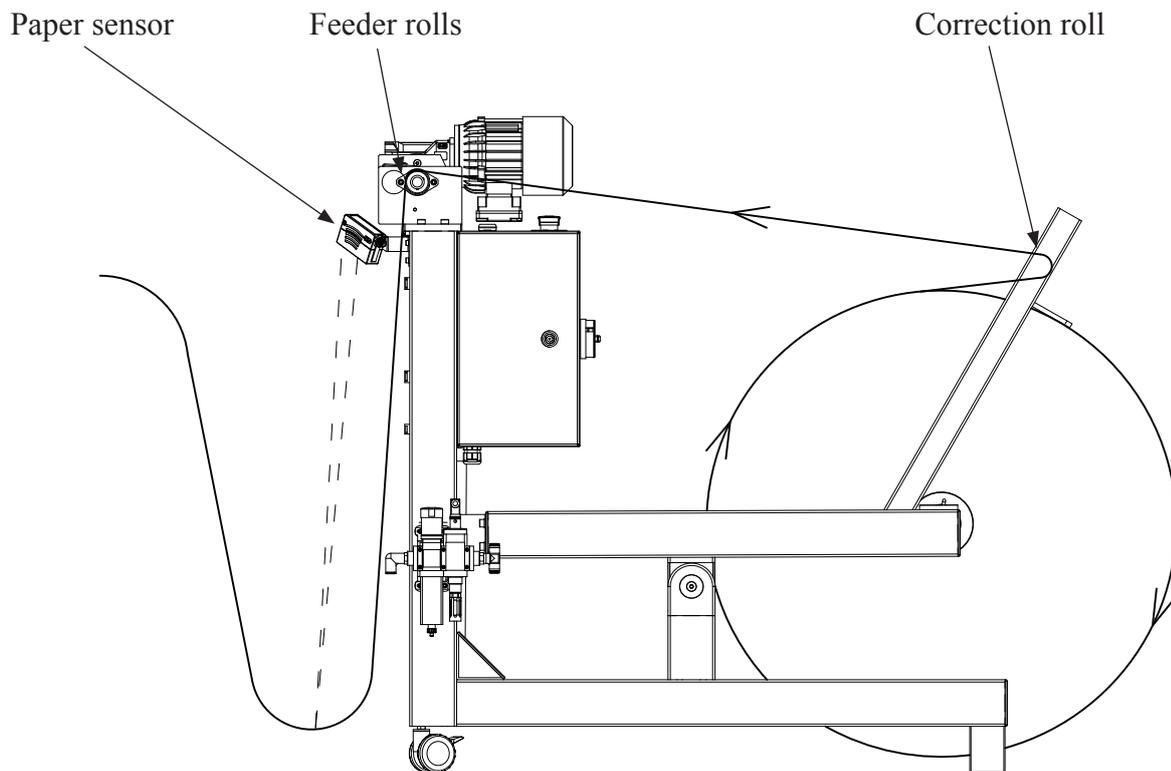
The paper sensor is a laser distance sensor, and is using a laser beam to check the distance to the paper. If the distance is long (the paper is close to the floor) feeding speed is slow (or it will stop completely) and if the distance is short, feeding speed is high. This will ensure that there is a constant slack of paper between the Paper Roll Feeder and the Printer.
