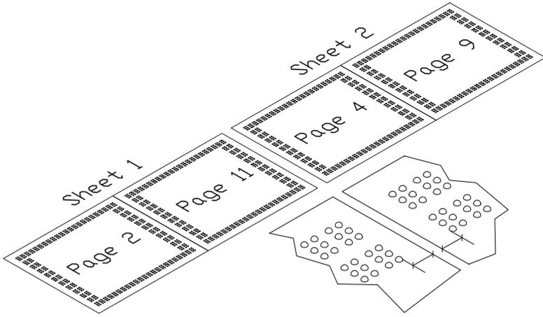
When the paper cutter is correctly adjusted, the right margin on page 11 has approximately the same size as the left margin on page 4. The edge on the sheet is also aligned with the text.
