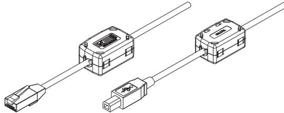
There is no need to select which of the two input to use. The Printer will connect to the input who receives data first. Meaning, if data comes on the ethernet, the USB will not be operative before the ethernet have finished the transmission.
