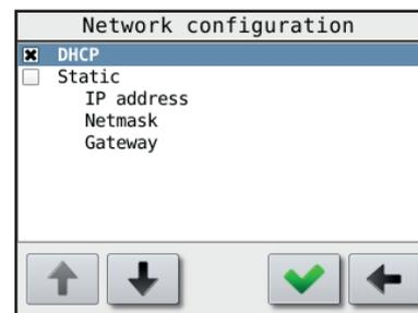
The three different settings for the static IP is set using the buttons as shown in the figure to the right. Type the numbers into the first text cell, then tap the next cell to move to it. When all four numbers are set, press the green **Accept** button to go back to the Network configuration menu.
