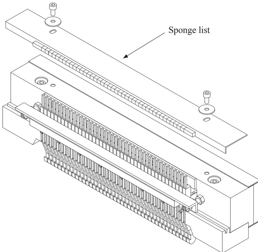
**Step 2.** Remove the two nuts holding the support list, and then remove the support list.
