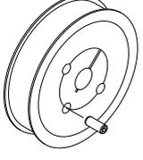
Place one of the screws in the third hole, and screw it inwards until the wheel is loose.
