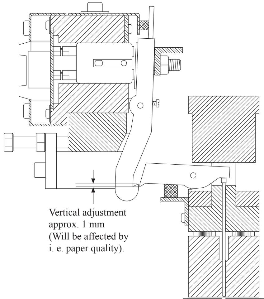
The vertical adjustment of the magnet rack sets the pressure of the printing pins when making dots.
