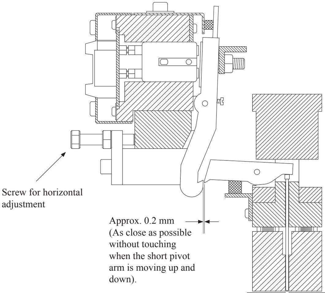
The gap between the long and the short pivot arm should be approximately 0.2 mm. When adjusting this, make sure that the gap is even for all the pivot arms and the same on both ends of the magnet rack.
