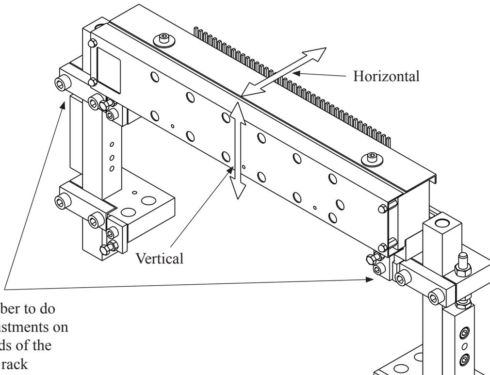
Remember to do the adjustments on both ends of the magnet rack
