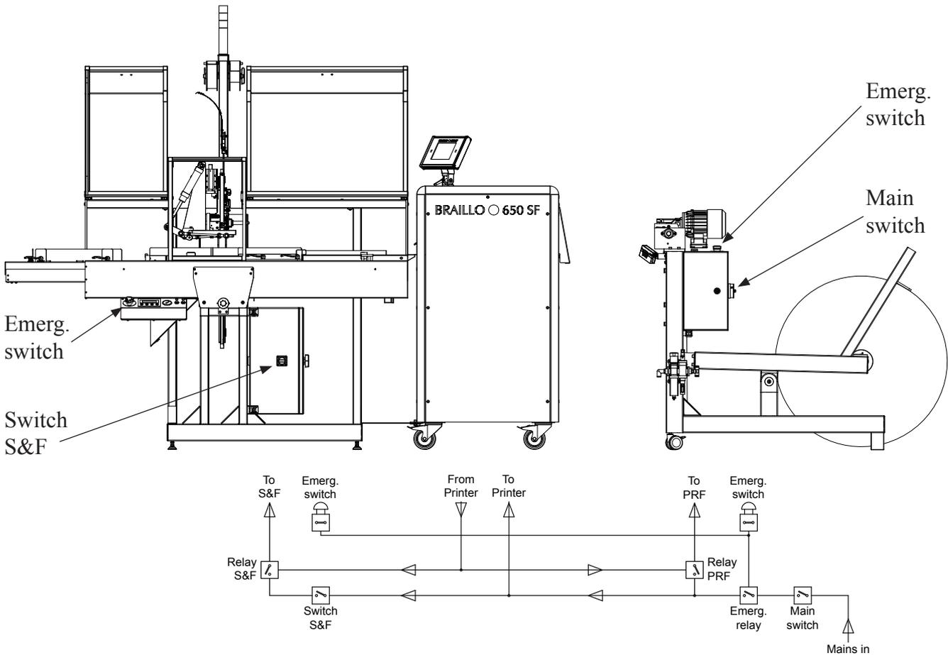
The way the units are connected regarding the 230 V is explained in the figure above. Please note that the emergency switches will turn off the power and air to all machines when they are pushed down. The main switch on the Paper Roll Feeder will also turn everything off.
