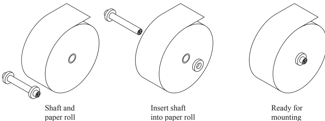
Put the shaft in the centre of the roll, and ensure that the shaft is approximately in the centre sideways. Fasten the shaft. The roll must be placed so that the paper is rolled off at the top. (See figure).
