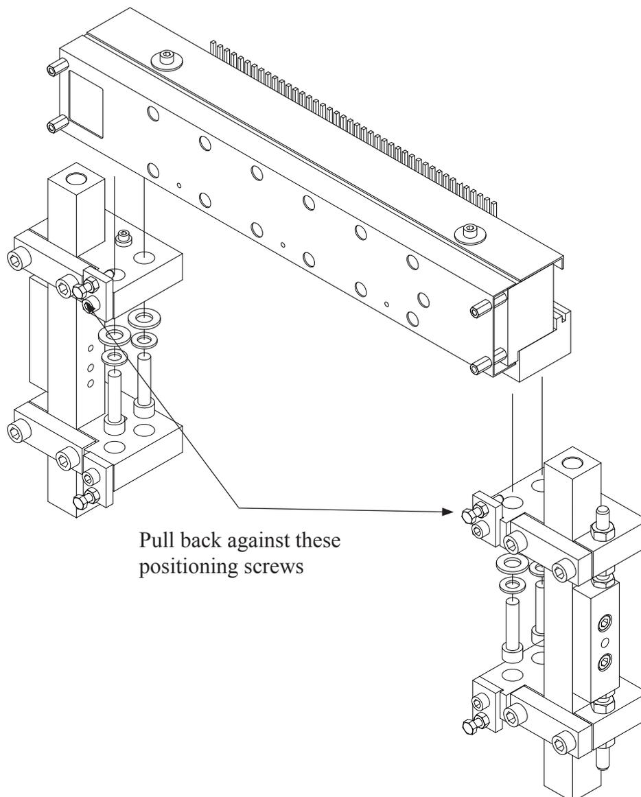
The magnet rack must be adjusted in two directions, horizontal and vertical. The horizontal adjustment is done first. This adjustment positions the magnet rack correctly in relation to the short pivot arms. If the Printer prints too many or too few dots, the horizontal adjustment could be the reason.
