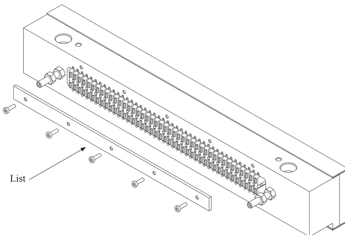
**Step 2.** Pull out the defect magnet with, e.g. a narrow pair of “needle nose” pliers.
