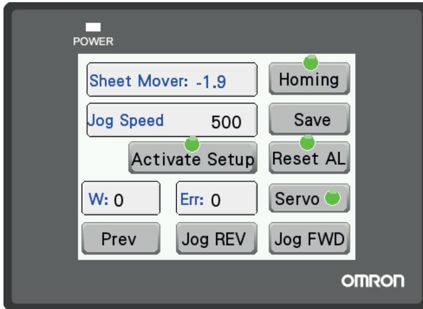
The arm that moves the paper or cover on the S&F unit must have a reference position to be able to position itself correctly when picking up or laying down paper.
