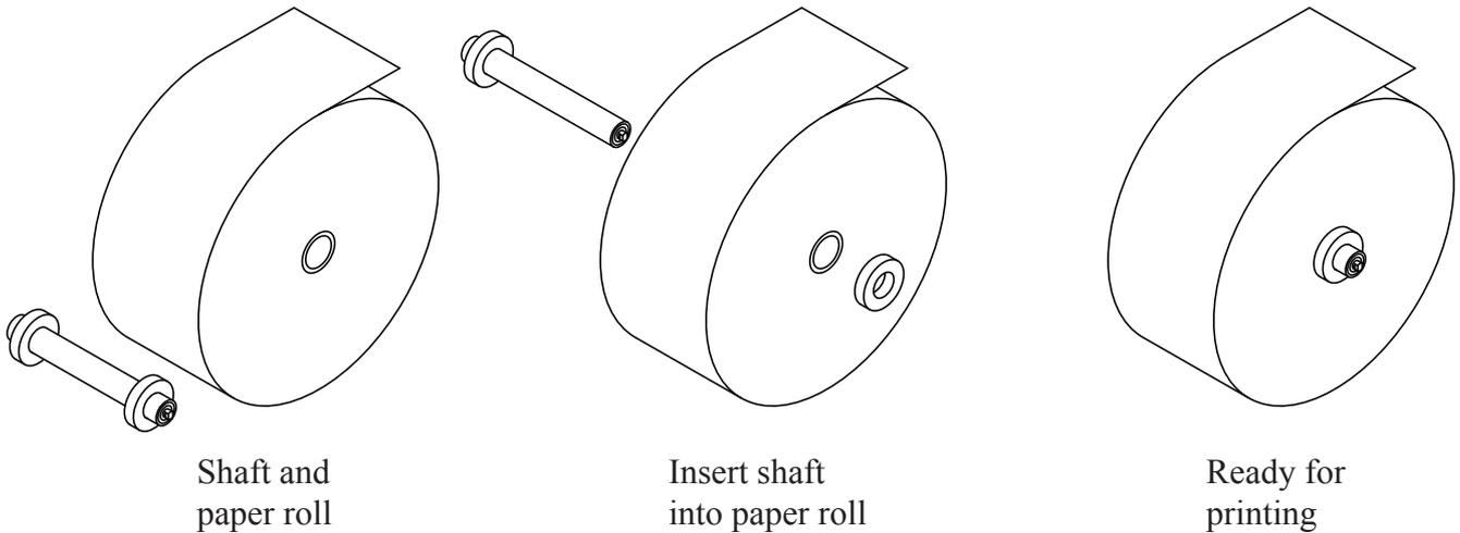
Put the shaft in the centre of the roll, and ensure that the shaft is approximately in the centre sideways. Fasten the shaft. The roll must be positioned so that the paper is rolled off at the top. (See figure).
