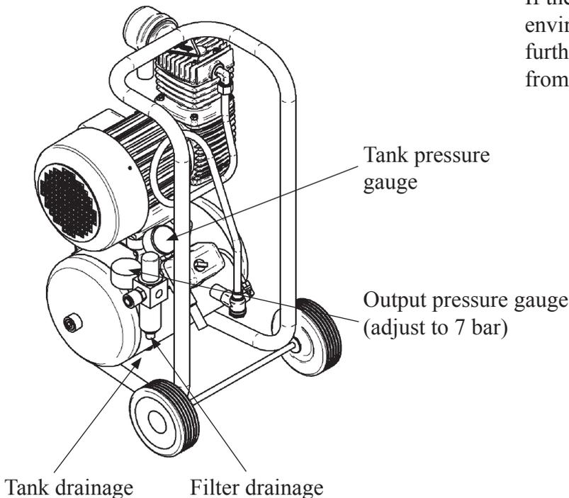
If the compressor is placed in a more harsh environment, it might be necessary to take further precautions to remove oil and water from the air.
