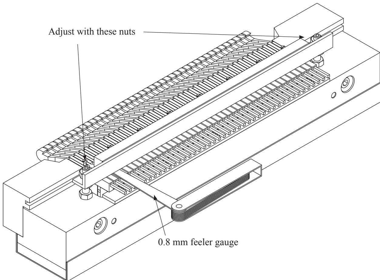
The second adjustment is the pressure the sponge list exerts against the pivot arms. The sponge list works as a return spring for the pivot arms. The correct adjustment is when the sponge list is slightly pressing against the pivot arms, but pivot arms still can move freely.
