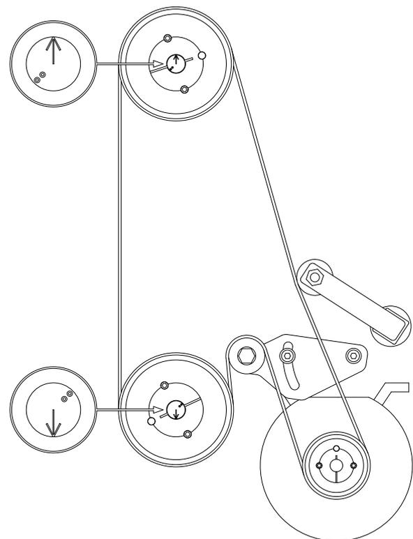
When the arrows at the end of the shafts are pointing in the opposite direction of each other, the short pivot arms will be positioned approximately like in the figure below:
