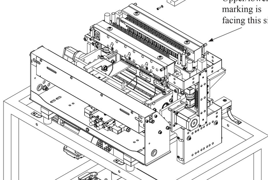
7. Now the beams and paper shoes can be lifted carefully upwards.
