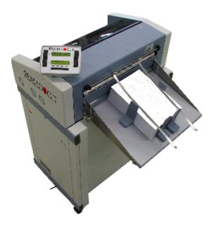
When it comes to bursting/cutting/trimming Braille paper, Braillo recommends the Braillo Cut 4, which is a modified Muller 6600 series forms cutter. This machine is made in Germany and is "Braille modified" in Norway. It is extremely reliable and Muller has over 45 years of experience with cutting/trimming continuous forms. The Braillo Cut offers users an attractive stand-alone option for cutting continuous Braille paper in a flexible and modular design.
